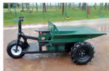
Electric Mechanical Cart: Assist in transporting and evacuation of FFB in the plantations
