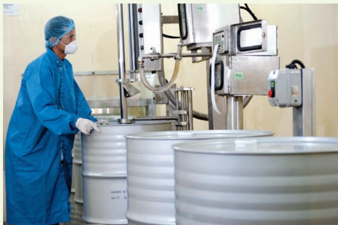
Refined glycerine is placed in drums in a GMP (good manufacturing practice) environment at IOI Oleochemical's manufacturing plant.
