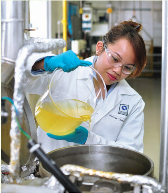
Sampling from the pilot perfector at IOI Loders Croklaan Asia is performed with meticulous care to check the shortening texture.
