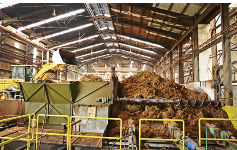
IOI's biomass co-gen power plant uses kernel shells and EFB to generate steam and electricity.
