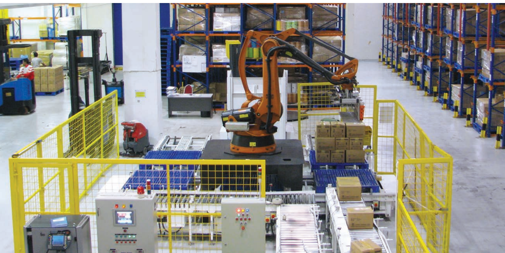
Below: The use of automatic robotic arm at IOI Lodars Crokiaan Asia, Pasir Gudang to stack packed cartons on pallets increases production efficiency.
