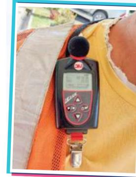
The workers wore the personal noise dosimeters for eight hours in order to determine their level of noise exposure as they worked.
